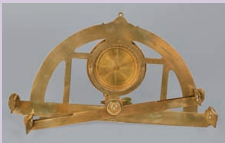
Figure 1. Graphometer made by Michael Butterfield, 1698
